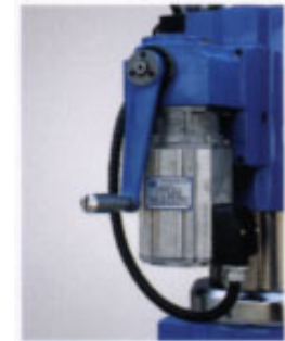
Lifting worktable by motor
