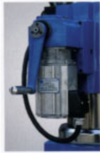
Lifting worktable by motor, manual
